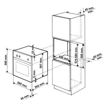
In order to ensure adequate ventilation, the back panel of the cabinet must be removed. Installing the oven so that it rests on two strips of wood is preferable. In the case where the oven rests on a continuous, flat surface, there must be an aperture of at least  $45 \times 560$  mm.
